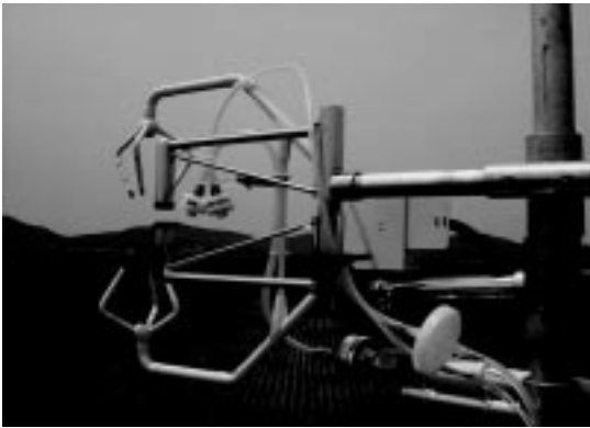
Fig. 1. The eddy covariance system used in measuring the water vapor flux.
